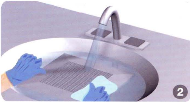
Wash and clean louver
