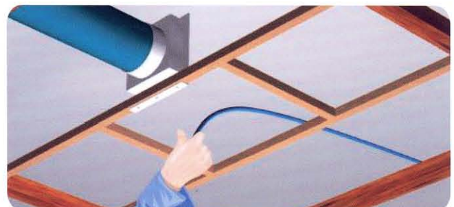
Pull power cord out of ceiling and insert into housing.
